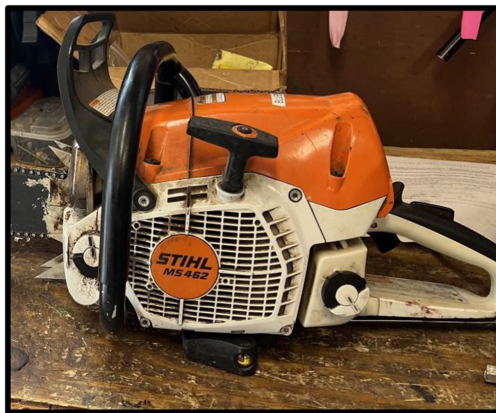
Photo 4: A Stihl MS 462 chainsaw. The fuel window (bottom, right) on a heavily used saw often gets dirty or degraded.
